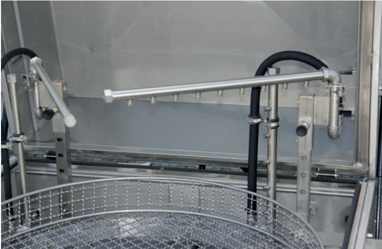
HTW Max Eco – Height-adjustable nozzle holder for cleaning and air shower
