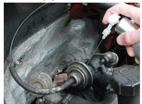
Cleaning an engine with AF Clean in the Air Force spray bottle
