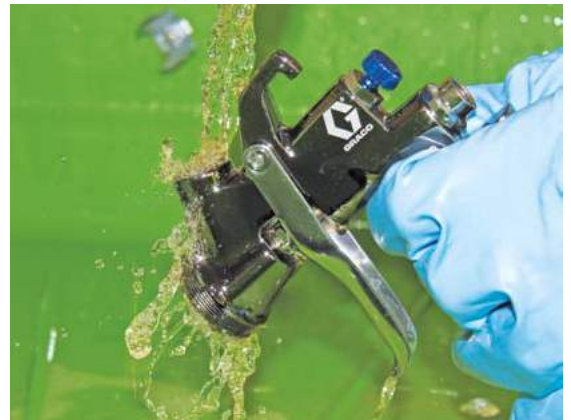
Cleaning of a spray gun in the PROLAQ Compact
