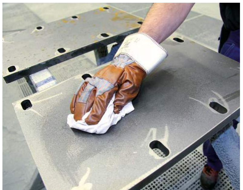
Cleaning before bonding
